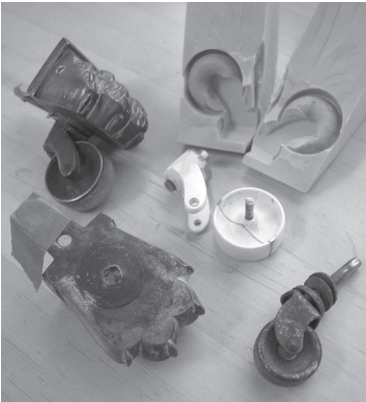
Figure 5. (left) Wheel and yoke, silicone rubber mold and polyurethane patterns for brass casting—to replace the modern wheel (lower right corner).
