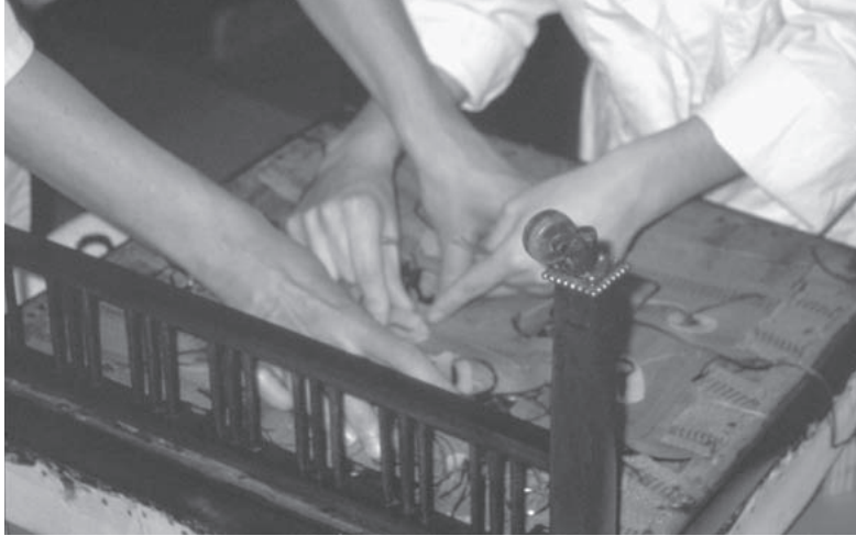
FIG. 3 It is helpful to have one person apply pressure to compress the springs while a second person ties the cords to hold the compressed height. Courtesy New York State Office of Parks, Recreation and Historic Preservation, Olana State Historic Site.
