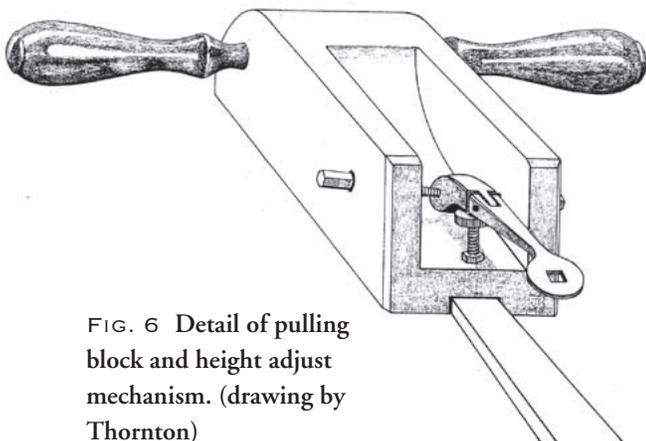
FIG. 6 Detail of pulling block and height adjust mechanism. (drawing by Thornton)
