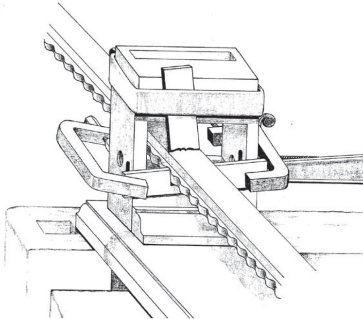
FIG. 7 Detail of cutter-head and slide-board clamped into the end-vice of a cabinet makers workbench. The device is set up to make a side-to-side (*flammeleisten*) waveform molding. (drawing by Thornton)
