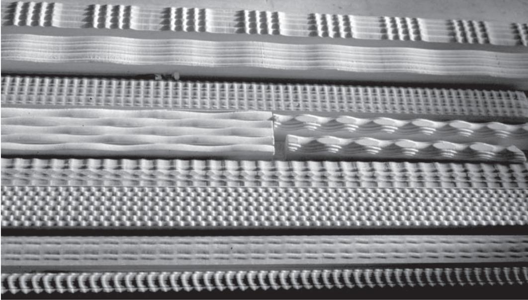
FIG. 9 A selection of moldings made on the Moxon “Waving Engine.”
