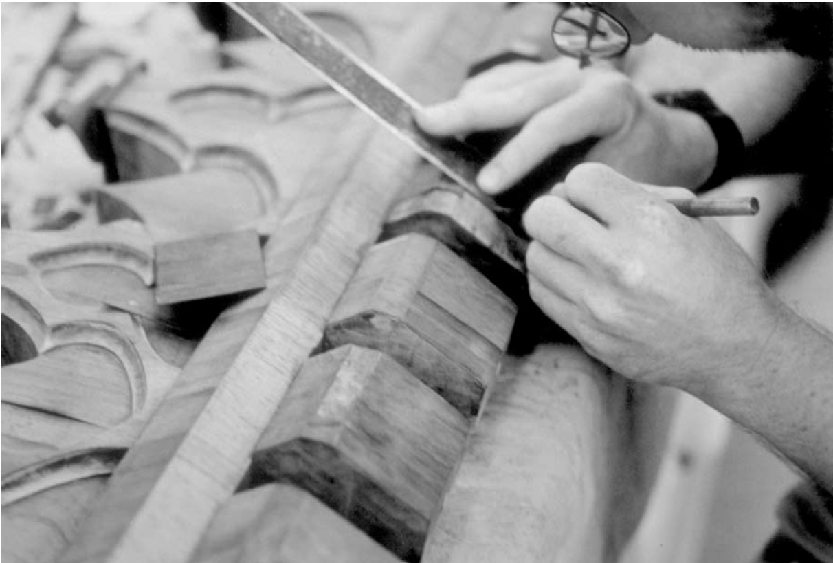
Replacing missing veneers with Brazilian rosewood.
