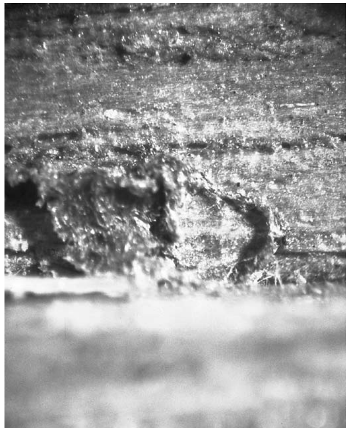
Figure 6: A fabric sample found along the cut lines around the sofa cushion rail containing blue and green mohair and cotton fibers.
