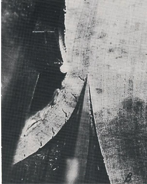
**Figure 7** Veneer slicing/introduction of knife checks
