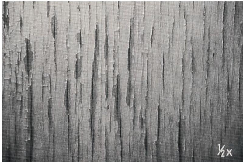
**Figure 8** Knife checking of plywood surface veneer
